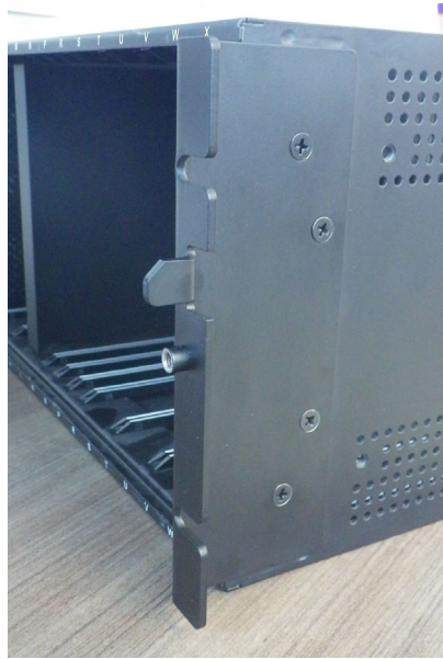
Figure 10-20: Attach mounting bracket to relay on right side
