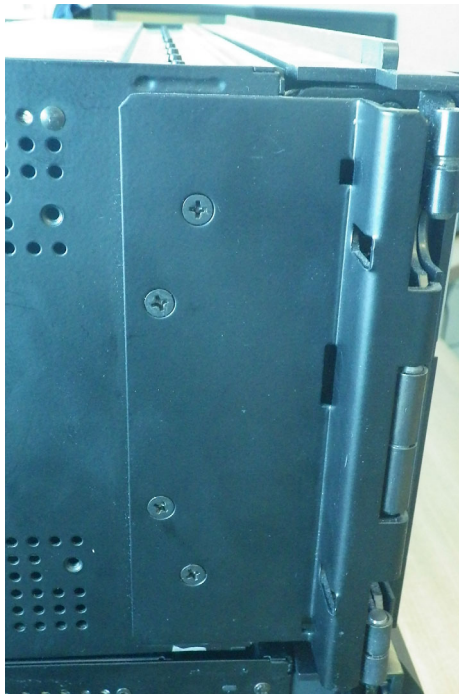
Figure 10-18: Unscrew basic front panel mounting bracket on left side
