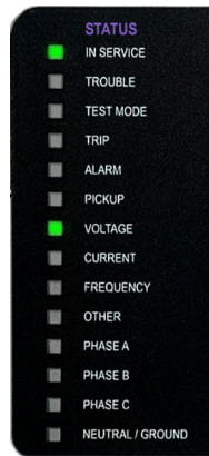
Figure 4-51: Example of LEDs on graphical front panel
