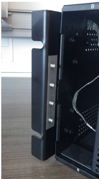
Figure 10-19: Attach mounting bracket to relay on left side (no power supply module in first slot)
