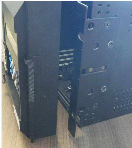
Figure 10-15: Remove basic front panel mounting bracket on right side
