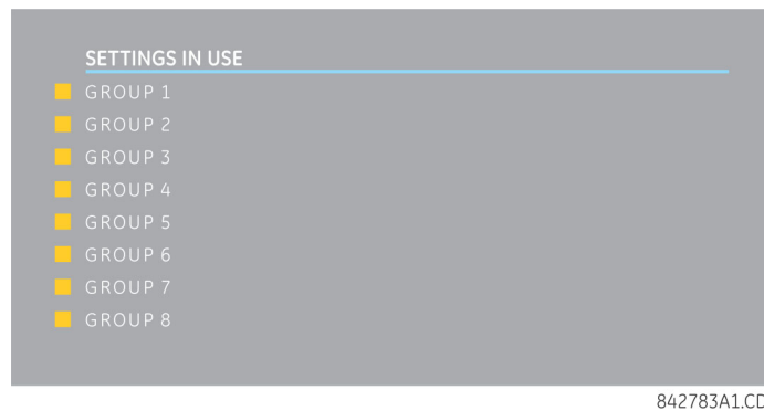
Figure 4-50: LED panel 2 (default labels)
