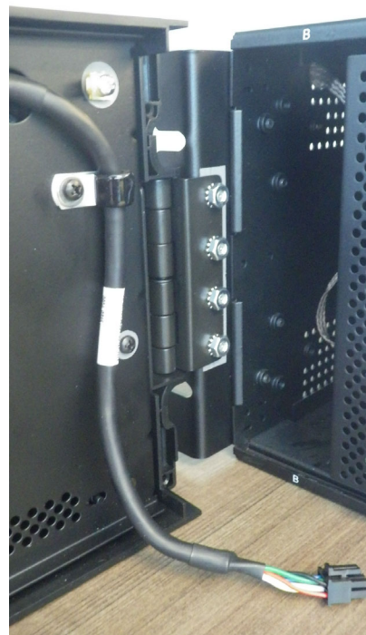
Figure 10-21: Attach to left mounting bracket inside relay
