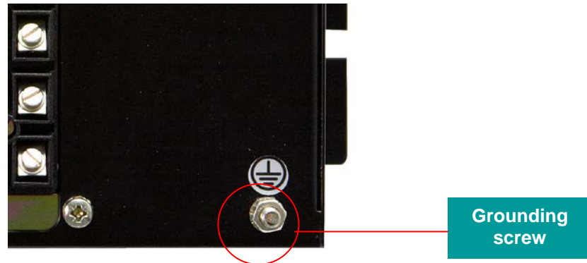
FIGURE 1-3 GROUNDING SCREW LOCATION
