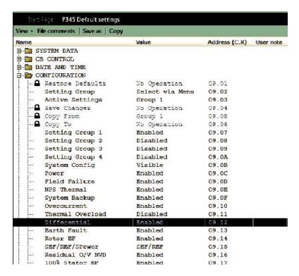
Figure 1 Simple function selection by mouseclick
