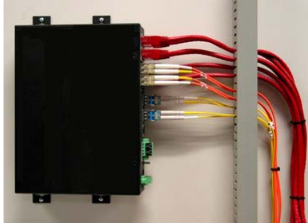
Figure 3-3: Typical Panel / Wall mounting of the ML810 Switch (position 2 shown)
