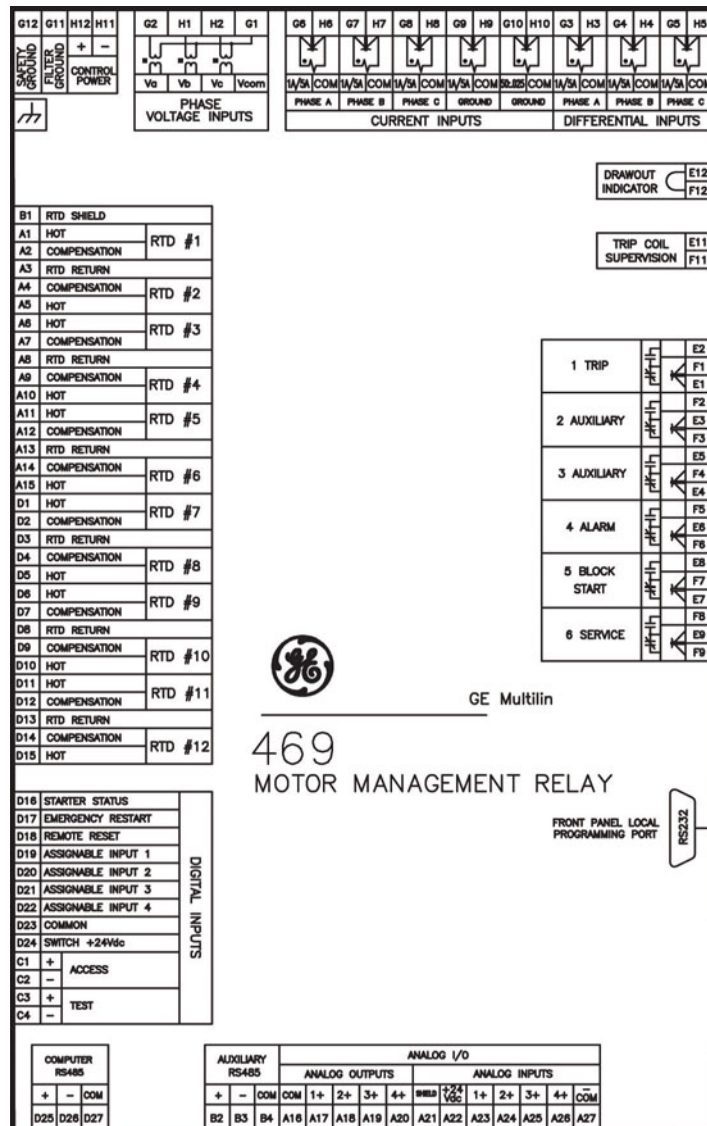
FIGURE 2-2: SR469 Terminal Functions Schematic
