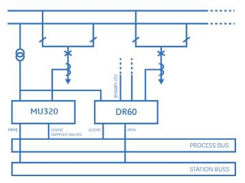
The DR60 can be used to translate the analog and binary signals into IEC 61850 standard protocol as GOOSE and MMS.
