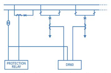
The DR60 can be installed to monitor and record analog and binary signals. Depending on the part number option, with a single DR60 it is possible to have: up to 32 analog inputs; up to 96 binary inputs; up to 32 high-speed transducer inputs for HVDC or up to 48 binary outputs.
