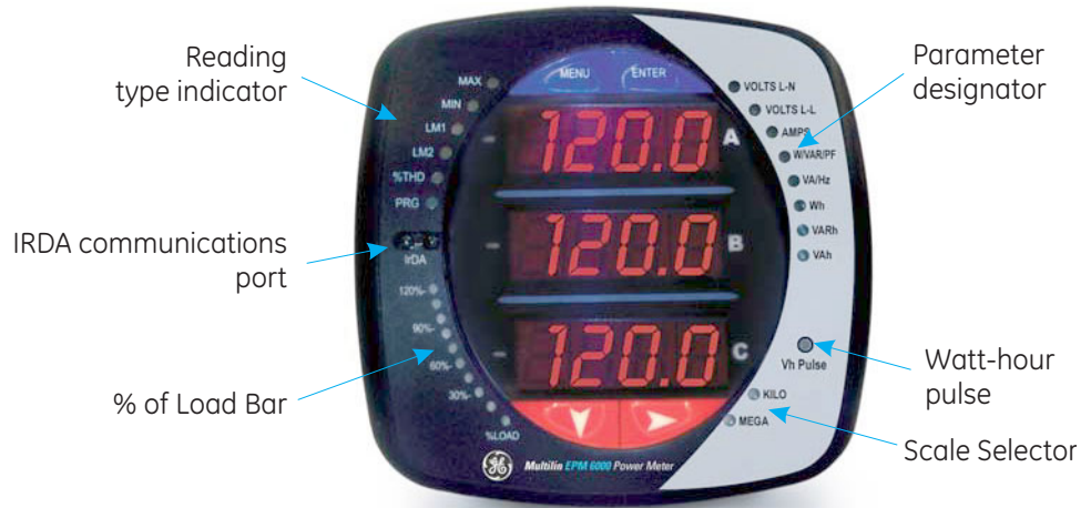
Figure 6-1: Faceplate of EPM 6000 Meter with Elements
