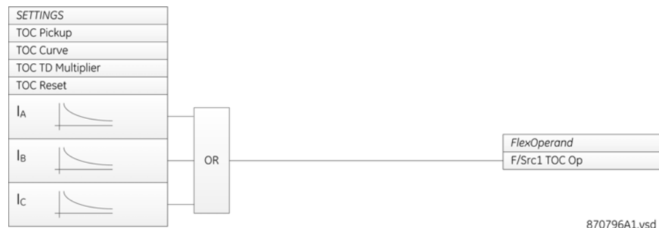
Figure 20: Bus sources inverse time overcurrent logic diagram
