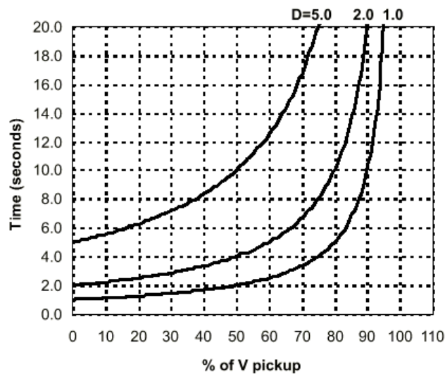
Figure 5-12: INVERSE TIME UNDERVOLTAGE CURVES
