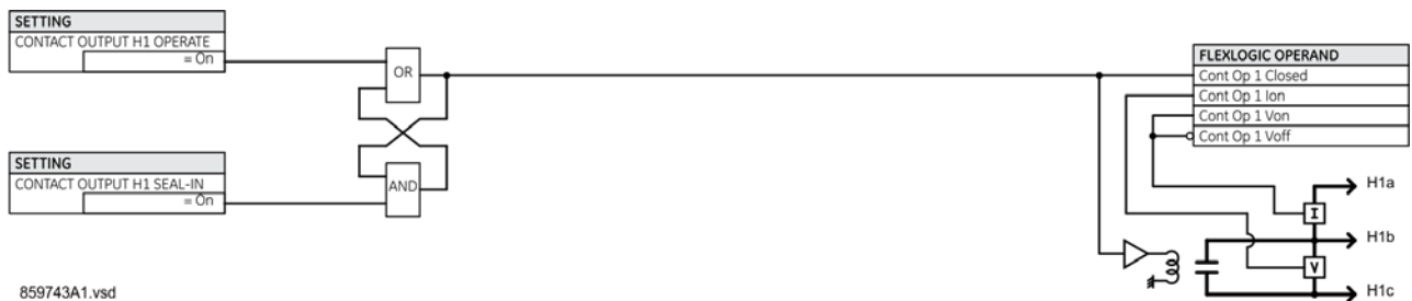
Figure 5-160: Contact input/output module type 6A contact 1 logic
