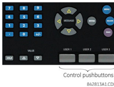
Figure 5-43: Control pushbuttons (enhanced faceplate)
