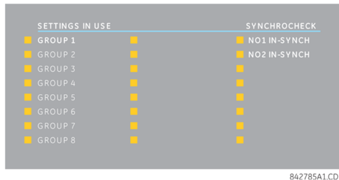
Figure 4-26: LED panel 2 (default labels)
