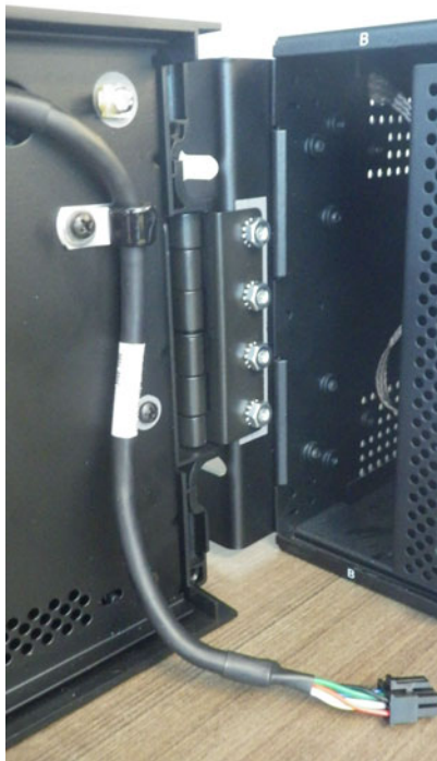
Figure 11-21: Attach to left mounting bracket inside relay
