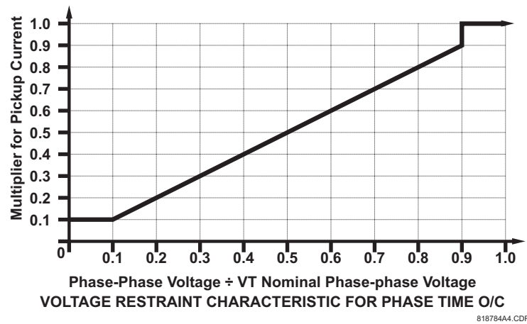
Figure 5-107: Phase time overcurrent voltage restraint characteristic
