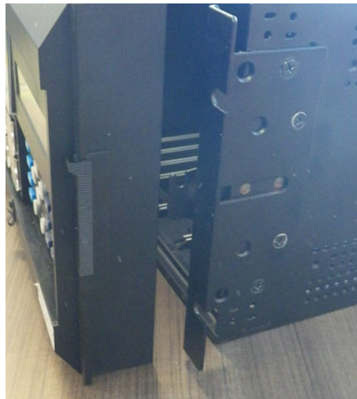
Figure 11-15: Remove basic front panel mounting bracket on right side
