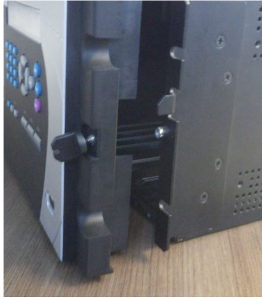
Figure 11-15: Remove basic front panel mounting bracket on right side
