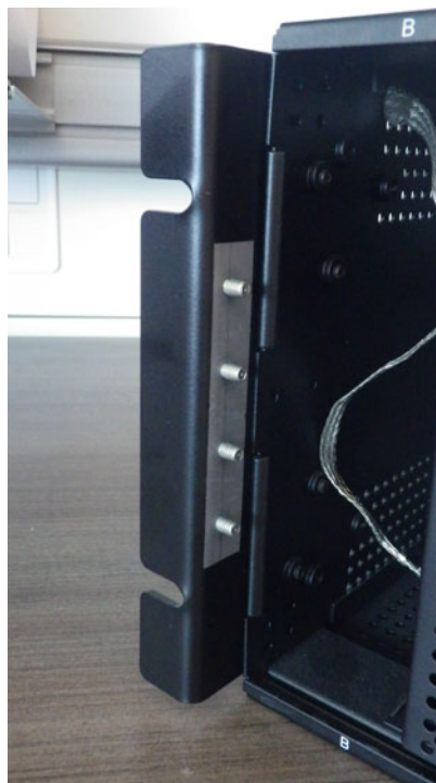
Figure 11-19: Attach mounting bracket to relay on left side (no power supply module in first slot)
