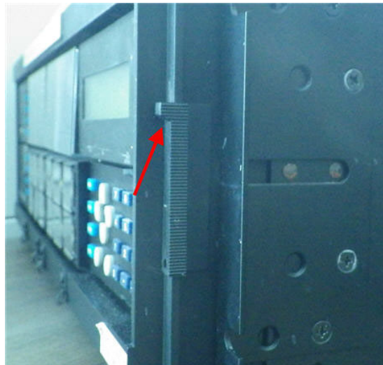
Figure 11-13: Lift latch on basic front panel to open
