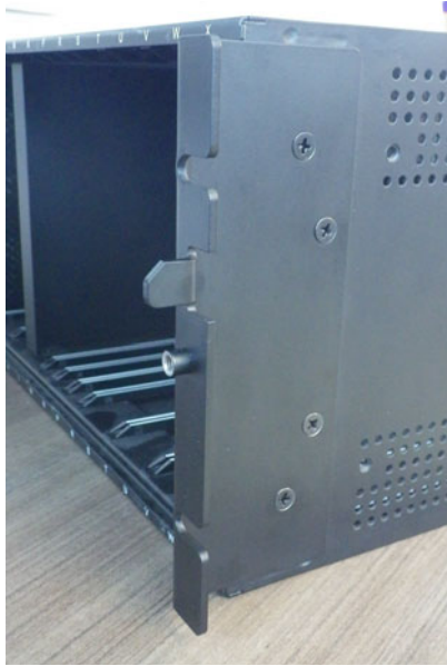
Figure 11-20: Attach mounting bracket to relay on right side
